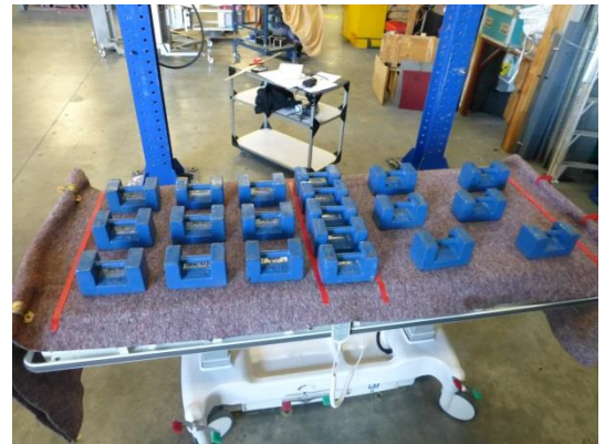
FIG.2 VERTICAL LOADING TEST SWL OF 200KG
