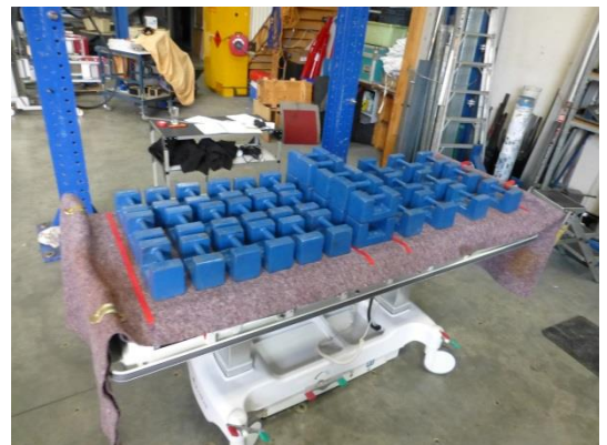
FIG.3 VERTICAL LOADING TEST 400KG
