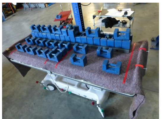
FIG.4 LATERAL STABILITY TEST
